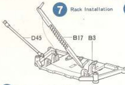
Fig. 7 - Rack Installation Fit B 17 and D 45 into bulkhead B 3.
