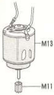
Fig. 21—Assembling Gear Box Put motor M 13 in gear box M 10 and fix it with screws 12. Check the gear box functions by connecting the motor leads to the battery.
